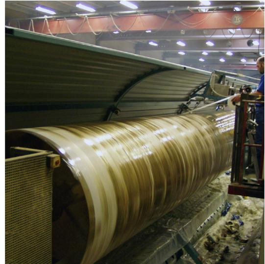
The stack liners were manufactured using Tunetanken's cutting-edge winding technology.
